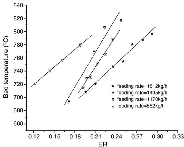
Fig. 3. Relationship of bed temperature and ER at different feeding rates.
