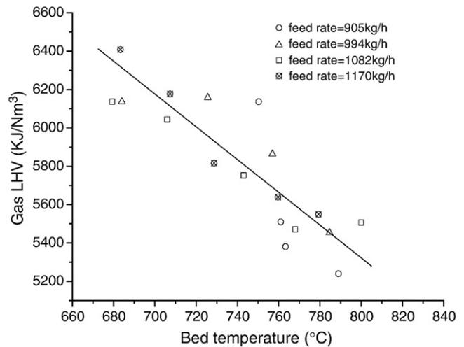
Fig. 4. Relationship between gas heating value and bed temperature at different feeding rates.
