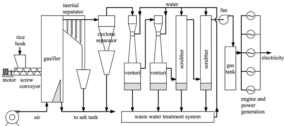
Fig. 1. Schematic of 1.2-MW rice husk gasification and power generation plant.
