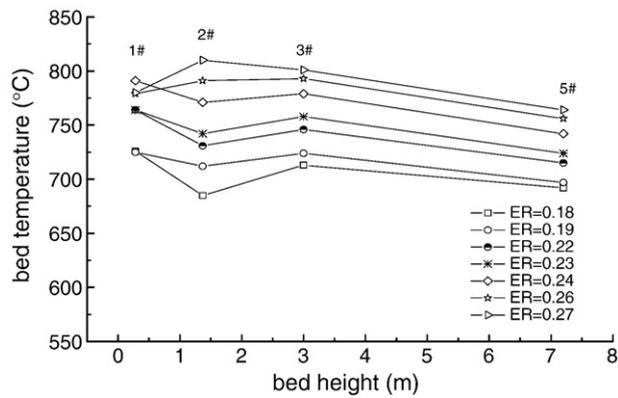
Fig. 2. Axial profile of gasifier temperature.
