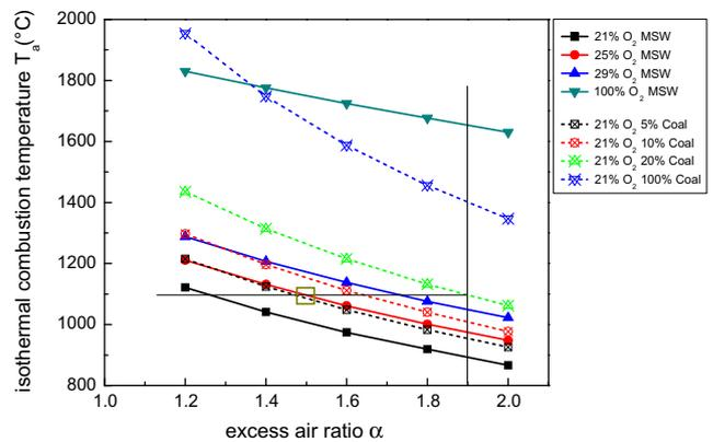
Fig. 2. Isothermal combustion temperature  $T_a$  of MSW incinerations with different coal proportions or oxygen concentrations.
