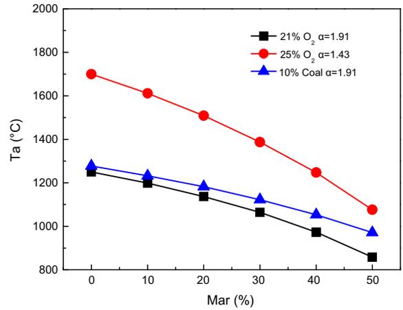
Fig. 5. Influence of moisture content in MSW on isothermal combustion temperature.
