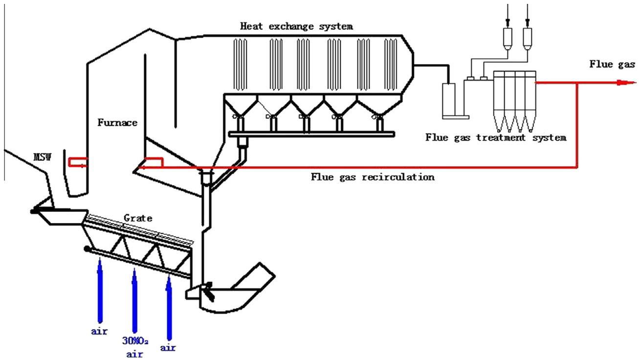
Fig. 1. Oxy-enriched incineration system of a grate furnace.
