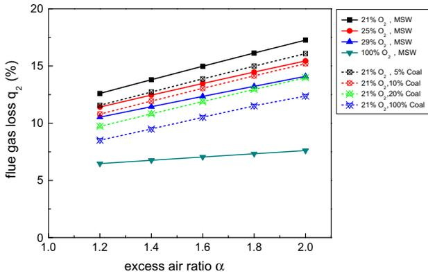
Fig. 3. Variation of flue gas loss under different combustion method in different excess air ratio.
