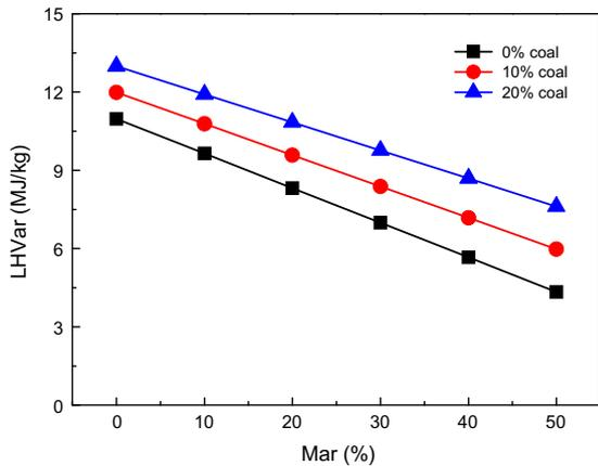
Fig. 4. Influence of moisture content in MSW on lower heating value of fuel.
