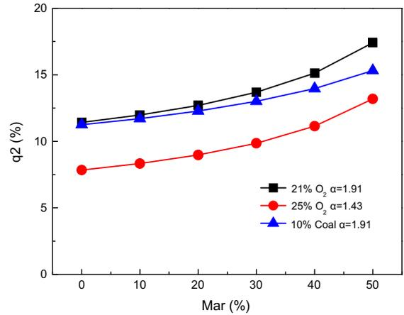
Fig. 6. Influence of moisture content in MSW on flue gas loss.
